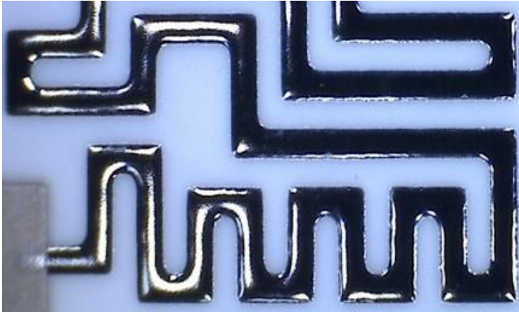
325-mesh screen, 20-mil Line/Gap Serpentine Ultra-High Ohm Value Resistor
