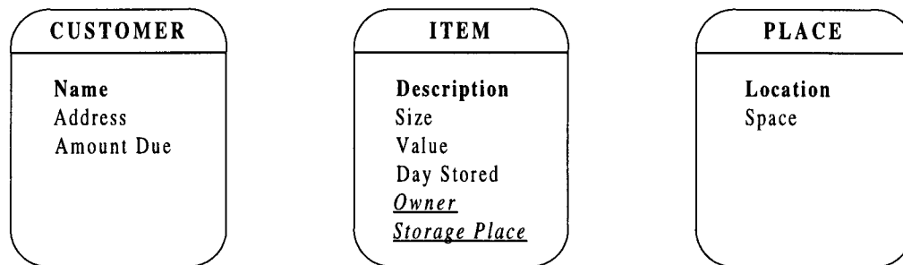
Figure 3.1. Three entities of the warehouse software [5]
