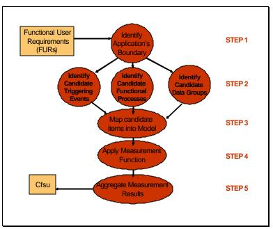
**Figure 3:** General procedure for measuring software size with the COSMIC-FFP method – ISO 19761
