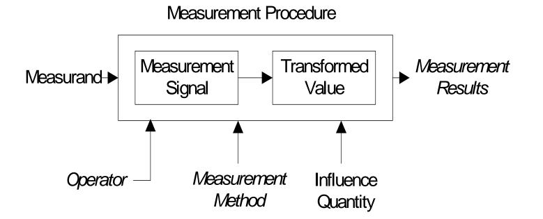
Figure 3: Measurement Procedure [ABRA02a]
