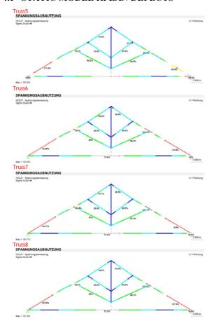
**Figure 6:** Structural models reporting decays and defects of the components (stress in the lower part of the rafters is generally a too high)
