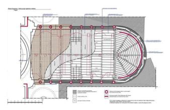
**Figure 9:** Plan of the presbytery-choir. Scheme of the restoration project for the roof structure.
