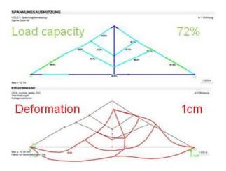
Figure 4: Results for the load case D-C (highest loads)
