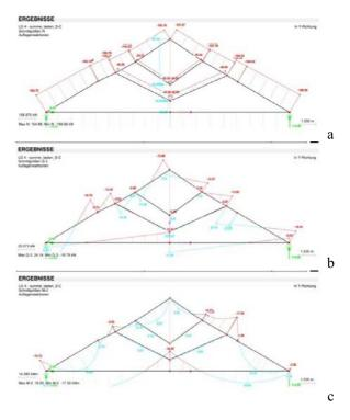
**Figure 5:** Axial force working on the beams (a); shear force working on the beams (b); axial force working on the beams (c).
