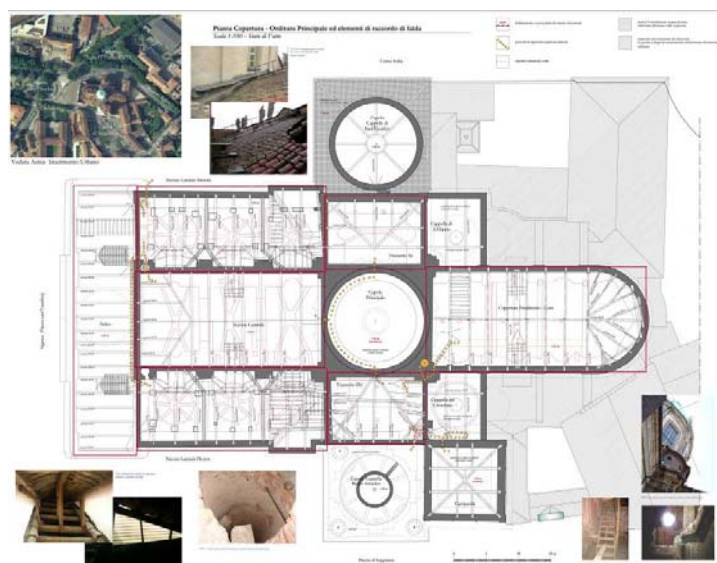
Figure 5: Plan of the timber roof structure
