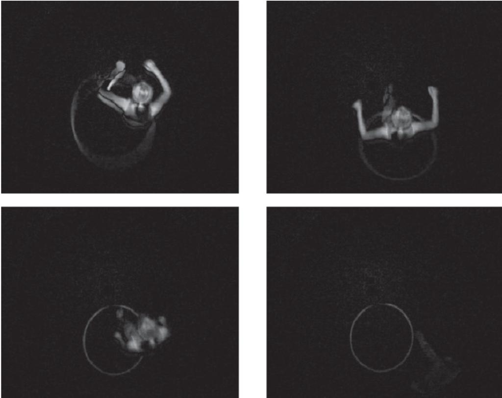
Figure 3-12. Greyscale images resulting from background subtraction with current frame and running average. Note the image is not binary but still contains 8 bits of information per pixel.
