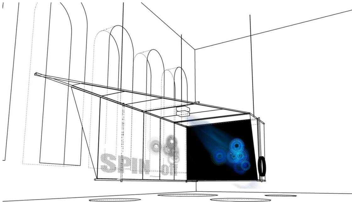
**Figure 3-4.** Sketch (to scale) of canopy frame, passive projection setup and the windowed side of the exhibition space.
