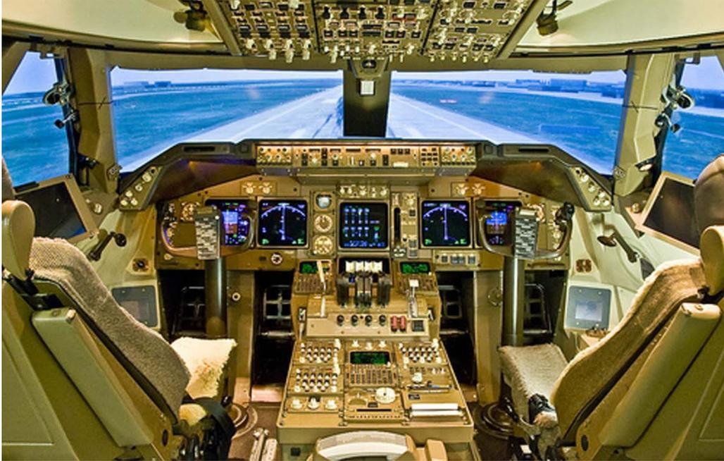
Figure 1-2. Image of a Boeing 747-400 Flight Simulator Cockpit.
