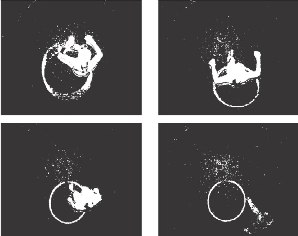
Figure 3-13. Thresholded binary image sequence resulting from the background subtracted imagery in Figure 3-12. Note the occurrence of noise due to light reflections incident on the floor interacting with the person.
