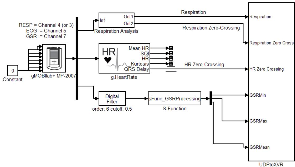
**Figure F-1. Simulink model developed for the Physiological Mirror. The leftmost block titled gMOBilab+ MP-2007 is the source where the raw signal is split up into respiration heart rate and GSR. For each of these a filter and analysis process exists in the middle. The data are combined again after analysis and transferred to the XVR program via UDP (right).**
