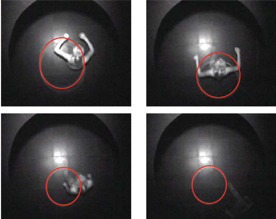
**Figure 3-14.** Detected Hough circles added into the original frame sequence. The algorithm does not always yield exact results as in the top-right frame for example. Instead it always yields the best fit given the data. Note that the algorithm is very robust although noise is present in the input images (c.f. Figure 3-13).
