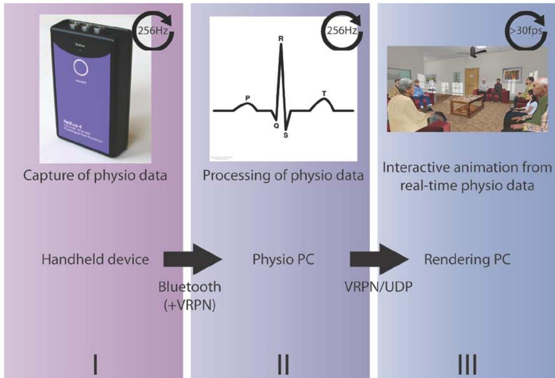
**Figure 4-18. Simple diagram of data flow and networking requirements. The left-hand block (I) is a device for capturing physiological data, which is transferred to a PC (II) via Bluetooth, where the data is processed. The resulting feature vector is then passed to another PC (III) where it is used to animate objects and the entire scene is rendered. Each block also shows the sampling or frame rate at which it operates.**
