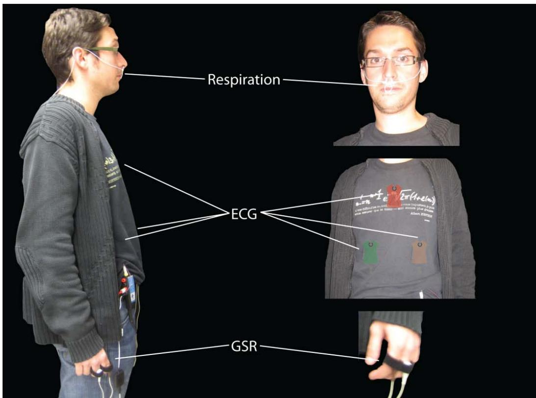
Figure 4-6. Front and detailed side view of a person wearing the three physiological sensors.
