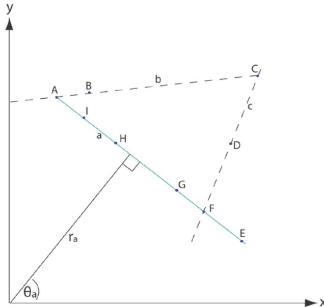
**Figure 3-10.** Given a number of points  $A$  through  $I$ , we can generate three lines with at least three of the points on them – in reality the Hough Transform evaluates many more possibilities. In Hough space the axes are not determined by  $(x, y)$  but in terms of the  $(r, \theta)$  parameters the line.
