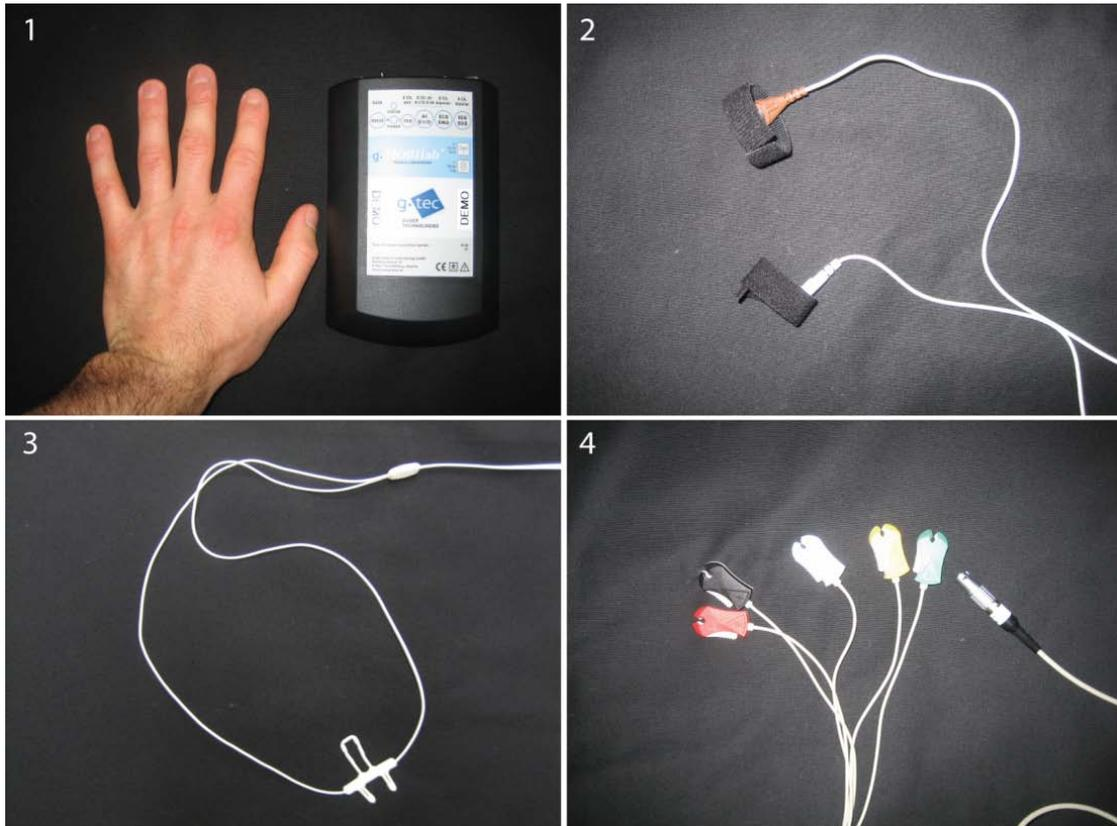
Figure 4-5. (1) Image of the wireless device used for physiological measurements. (2) GSR sensor attached to index and middle fingers, (3) Respiration sensor worn around nose and mouth, (4) ECG sensor, each of the five sensors are attached to various locations across chest and lower arm.
