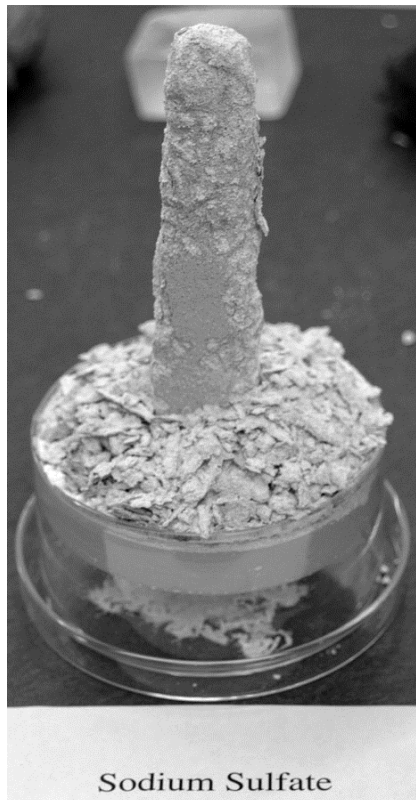
Figure 11. Bath limestone after exposure to 20% solution of sodium sulfate in high air exchange environment (10x/hr), 3 months. Note contour scaling. Note scales at base.
