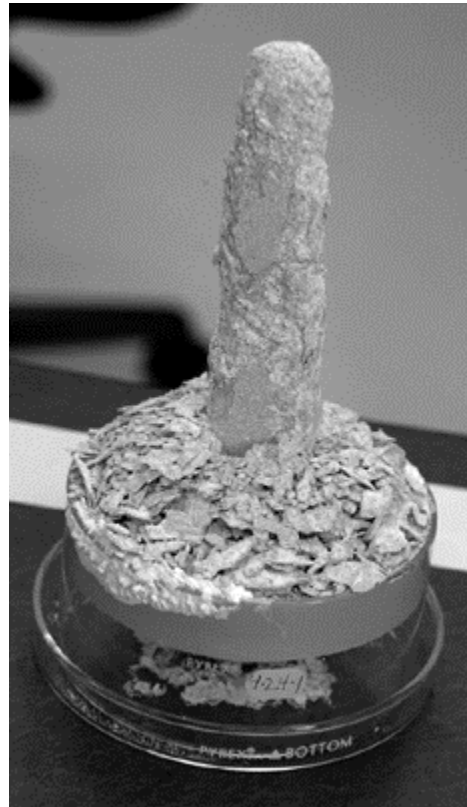
Figure 12. Opposite side of Bath limestone block after exposure to 20% solution of sodium sulfate in high air exchange environment (10x/hr). Note pile of scales at base of sample.
