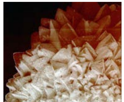
An electron micrograph of calcite crystals in a block of travertine stone. Photo: Eric Doehne.
