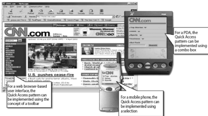
Figure 7: The Web Convenient Toolbar Pattern Implementations and Look & Feels for Different Platforms
