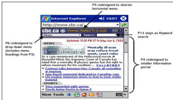
Figure 9: Migration of the CBC site to a PDA Platform using Pattern Mapping
