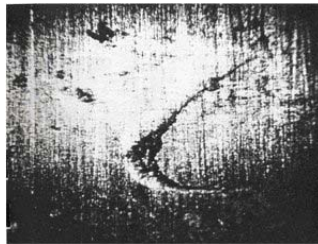
Fig. 79: Defect of 2-3 mm (shell or fish scaling) – 100Cr6 (Ascometal)
