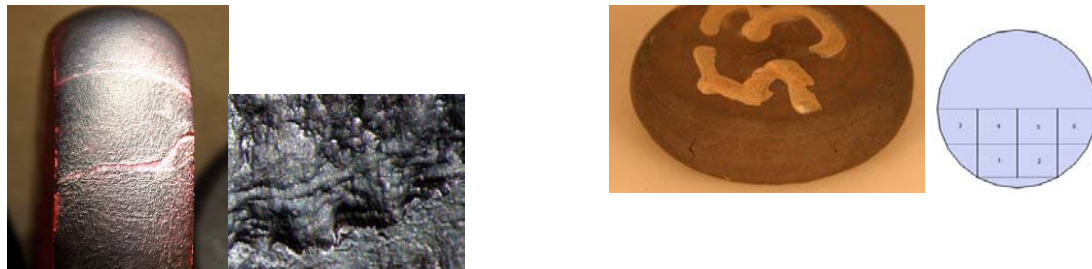
Fig. 114(a and b): (a) Rock drill upsetting compression trials – case 2 (b) dual phase higher sulphur (Mefos)
