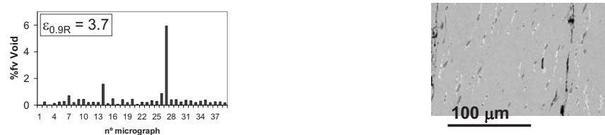
Fig. 134: Evolution of void volume fraction at increasing strain levels in as-cast steel LFCS 1/05 ext (CEIT)
