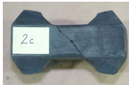
Fig. 7: Large scale deformed Corus RPS specimen (cooled side) (Mefos)
