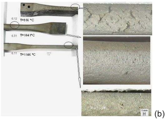
Fig. 10(a and b): crack opening after 60% reduction function of (a) remove cortical depth hc at T = 960°C (b) temperature for fixed hc = 13 mm 9SMn28 steel (CSM)
