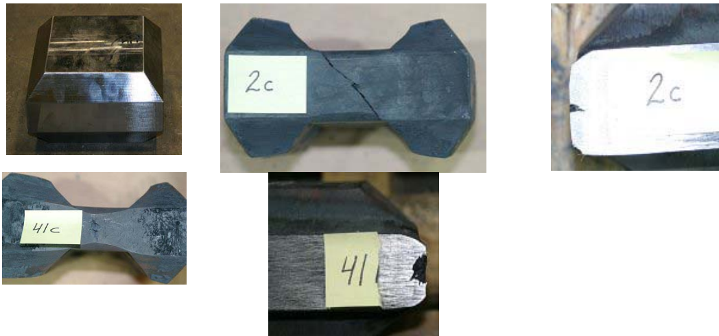
Fig. 115(a-e): (a) RPS large scale specimen (b, c) front and length cut Piece 2 (d,e) front and length cut Piece 41 - rock drill 4HS64 (Mefos)
