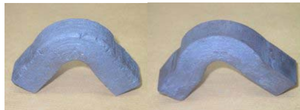
Fig. 89: (left) 3-point bending cracking of oscillation mark (hook type) – (right) Damage at corner and subsurface (no cracking)
