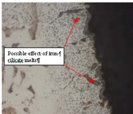
Fig. 30: FCS voided structure (tensile) with limited coalescence (Corus-Birmingham)
