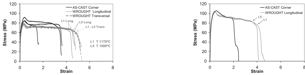
Fig. 106: Comparison of ductility between as-cast and wrought state at different positions at 1 \text{ s}^{-1}
