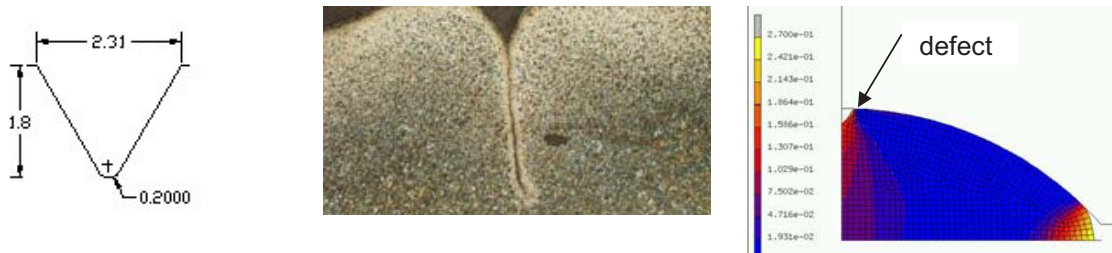
Fig. 122(a and b): (a) Artificial V crack on round bars rolled at Mefos in two passes (b) final crack after two passes (c) FEM damage (CL) after first pass
