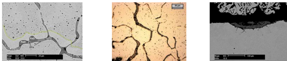
Fig. 146: Example of oxide and inclusions network on the surface of 9SMn28 (left) and LFCS steel (middle) and 9SMnPb30 (right) (FeS inclusions are clearly identified in the network) (CEIT)
