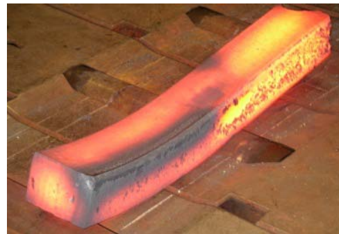
Fig. 5: hook type oscillation and Mn depletion (Sidenor, CEIT)
