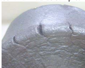
Fig. 89: (left) 3-point bending cracking of oscillation mark (hook type) – (right) Damage at corner and subsurface (no cracking)
