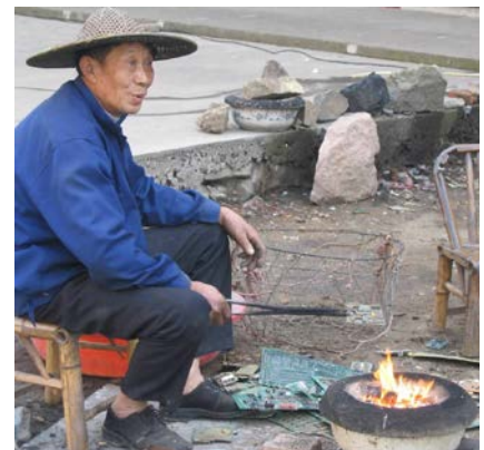
Figure 1: Typical recycling processes applied in the informal sector of developing countries (open burning of cables, leaching of gold from PWB, desoldering of PWB)
