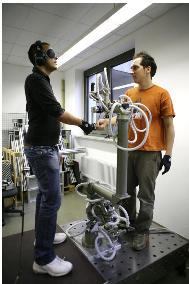
Fig. 5. The experimenter performing a 'human' s-handshake with a participant 'through' the robot.
