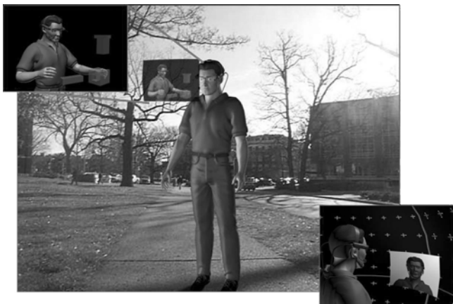
Figure 1 Conceptual drawing of the application scenario enabled by the Teleportal System. Two distant users are interacting on a task. One user is instructing how to proceed from a mobile location, while the other is executing the task. Both have visual feedback of the other's environment.
