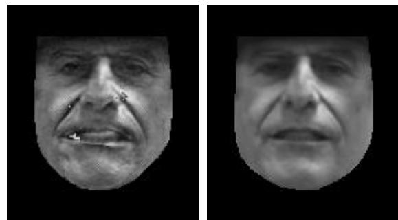
Figure 8 Outlier Effect on LS. It is shown how LS1 (left) is more susceptible to outlier effects than RLS1 (right).
