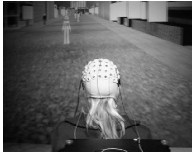
Figure 2: Participant in the virtual main street with shops and animated avatars during the Cave-FB. The subject wears an electrode cap (connected to the amplifier) and shutter glasses.
