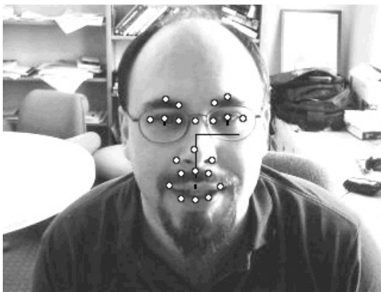
Figure 3: The 22 anchor points automatically tracked without using facial markers by the Nevenvision Facial Feature Tracker at 30 Hz.
