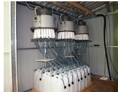
Fig. 2. Automatic sampler (a.k.a. Octopus sampler) setup with 24 x 20 L HDPE bottles in a tailor-made shed.
