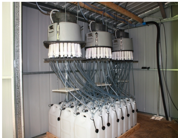
Figure 2: Automatic sampler (a.k.a. Octopus sampler) setup with 24 x 20 L HDPE bottles in a tailor-made shed.
