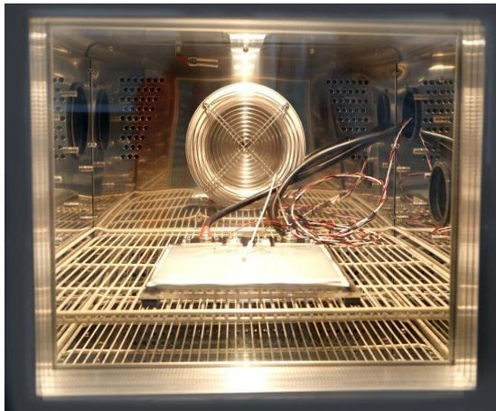
Figure 1: Snapshot the cell tested inside Memmert TTC 256 temperature chamber
