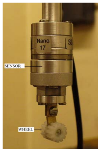
Fig. 2. Structure of the cylindrical wheel-based force sensor.
