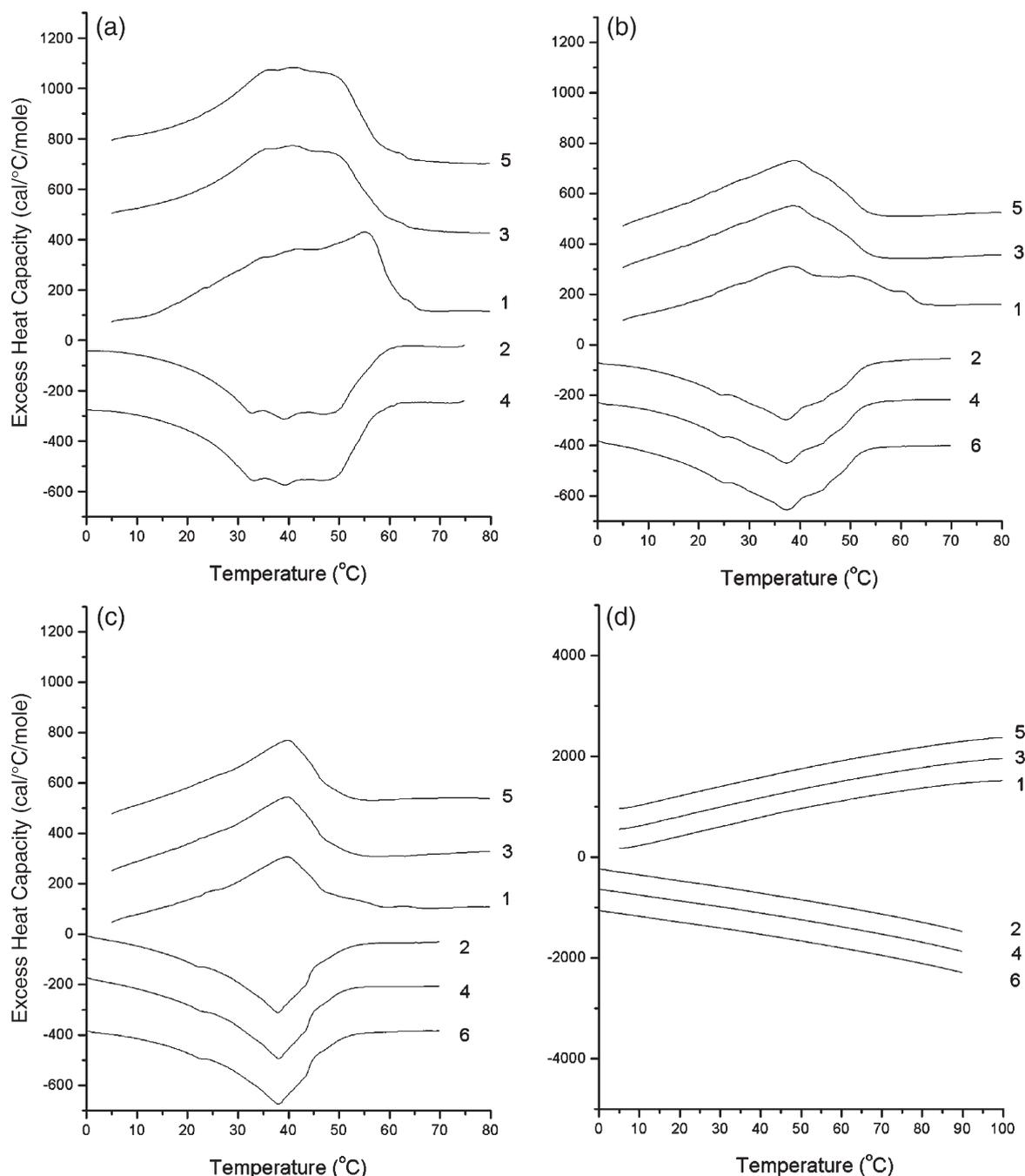
**Figure 3.** DSC heating and cooling curves for DPPE:CL (0.65:0.35, mol:mol) with added cytochrome *c* at a lipid to protein molar ratio of (a) 200, (b) 430, and (c) 870. (d) CL with added cytochrome *c* and CL at a lipid to protein molar ratio of 200 as in (a). Other details are as for Figure 1.
